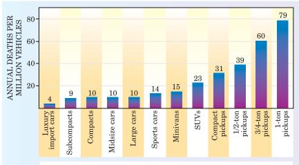
**Figure 6. Death risk for drivers** of the struck car in front-to-side impacts, shown as a function of the type of vehicle whose front struck the driver's side and normalized to the registered number (model years 1997–2001) of each type. (Data from Fatality Analysis Reporting System.)
