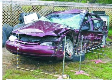
Figure 1. A midsize car struck on the side by a car of similar size suffered severe intrusion into the passenger compartment. In a study of traffic crashes at the University of Michigan, a measuring system determines horizontal deformations of the car relative to its original surface. As described in the article, the analysis of such actual road accidents, together with laboratory test crashes, provides guidance for safer vehicle design. (Photo courtesy of Joel MacWilliams.)
