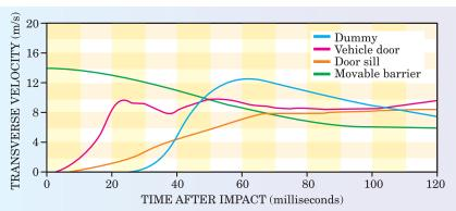
**Figure 4.** In a side-impact crash test, a moving barrier (green curve) strikes the driver's door of a stationary car at right angles at 31 mph, and then decelerates smoothly to 15 mph. The sill (orange curve) below the door roughly corresponds to the resulting lateral motion of the car as a whole. The rapid intrusion of struck door (red) into the passenger compartment propels the dummy driver (blue) to the right. The maximum acceleration of the dummy's bottom is 70g. (Adapted from ref. 5.)
