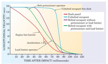
**Figure 3. Velocity history of a dummy** in the front passenger seat of a car, with various belt restraints, in a 35-mph head-on test crash with a fixed barrier. The red, leftmost curve, representing the car's dash panel, has a maximum deceleration of 27g about 60 milliseconds after impact.
