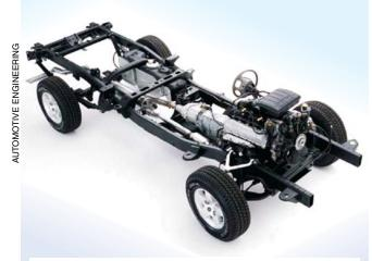
Figure 7. Half-ton 2002 Dodge Ram pickup truck. Its high, stiff horizontal rails are dangerous to the opposing vehicle in a crash. Such rails are typical of the body-onframe construction of most light trucks, in which the separately built passenger cabin and perhaps a cargo bed are welded onto a stiff chassis.
